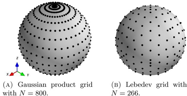
FIGURE 1. Distribution of nodes for Gauss quadratures.
